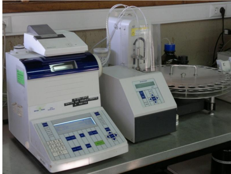
Figure 4.9: Digital density analyzer used, Mettler Toledo Density Meter De40 (ASTM Standards D5002, 2005).
