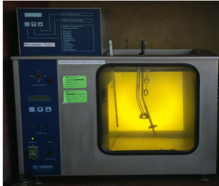
Figure 4.2: Viscosity Tamson bath with a viscometer for transparent liquids (ASTM Standards D445, 2009).
