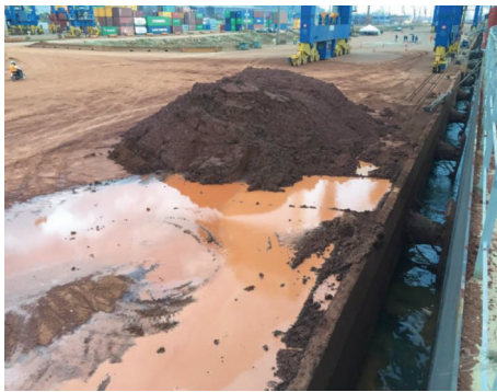
FIGURE 29: Bauxite cargo quayside exposed to the elements. Photo taken from the Medi Okinawa at Port of Kuantan, Malaysia [28].
