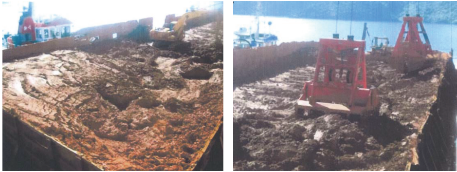
FIGURE 15: Photographs submitted to the head office by the Master of the condition of the nickel ore cargo at the time of loading at Kolonodale, Indonesia [26].
