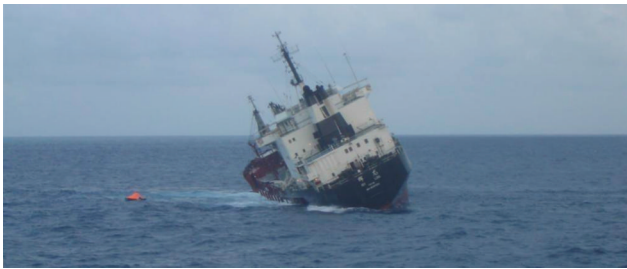
FIGURE 8: Hui Long listing severely to port after suspected liquefaction of the cargo of Fluorspar [29].
