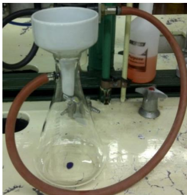
Figure 7: Vacuum filtration technique
