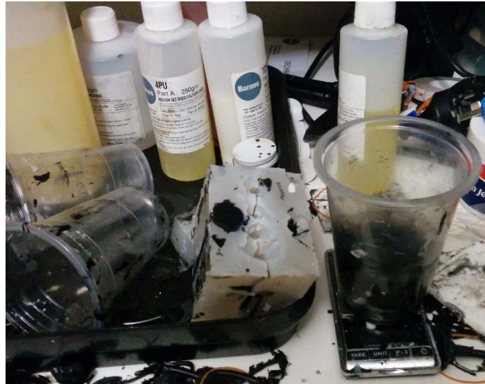
Figure 72: Silicone tooling and polyurethane resins for the ProxiMic
