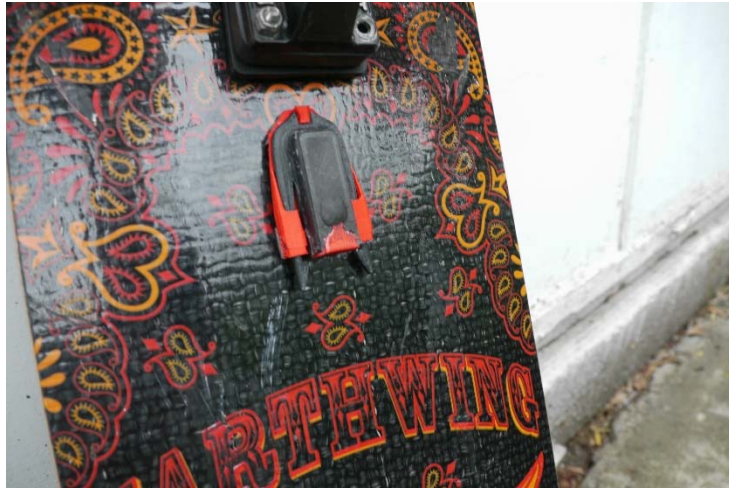
Figure 62 : The Surface microphone, mounted to the bottom of a skateboard
