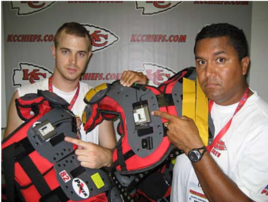
Figure 16: NFL films, wireless audio transmitters on pads 142
