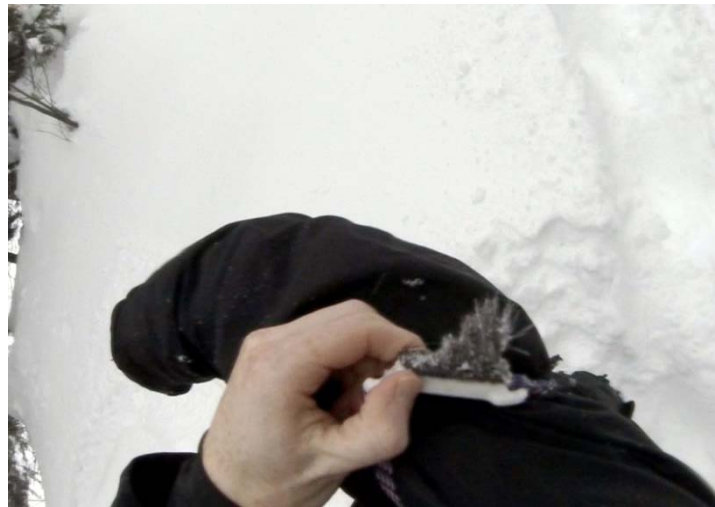
Figure 60: strap microphone placed on upper arm, snowboarding
