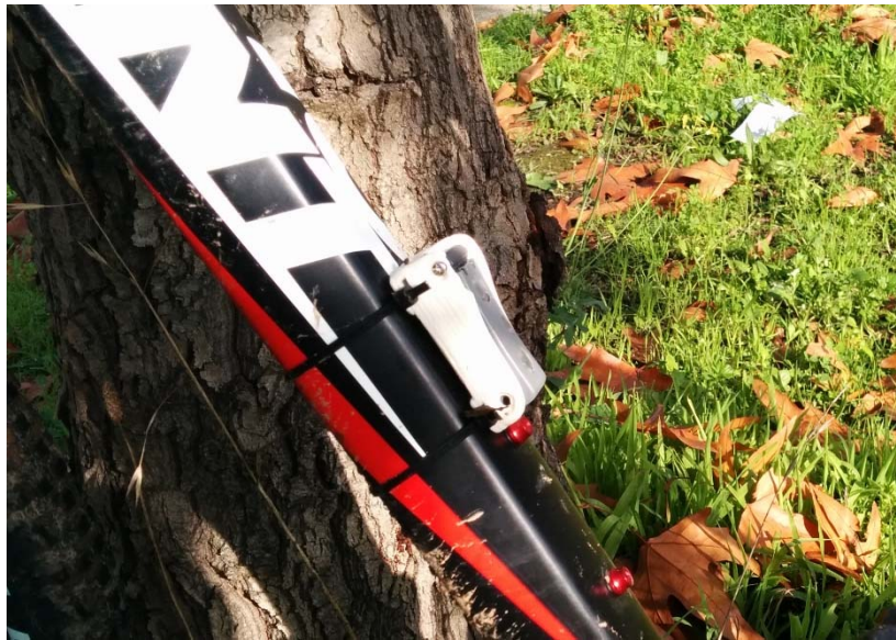
Figure 81: ProxiMic v3 equipment mount on bike
