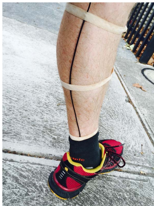
Figure 42: Footstrike microphones and wire placement
