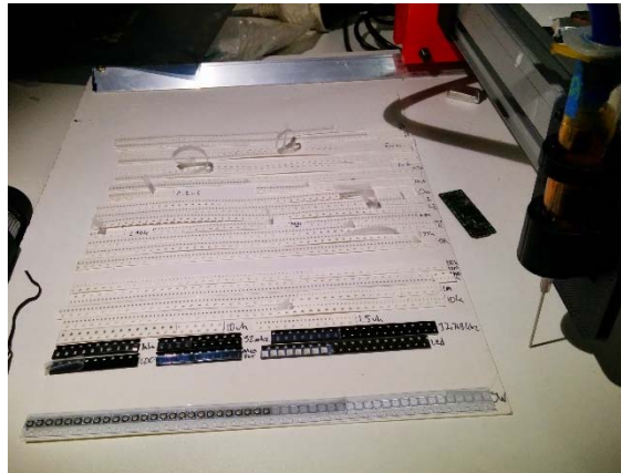
Figure 70: Manual pick-and-place circuit assembly machine
