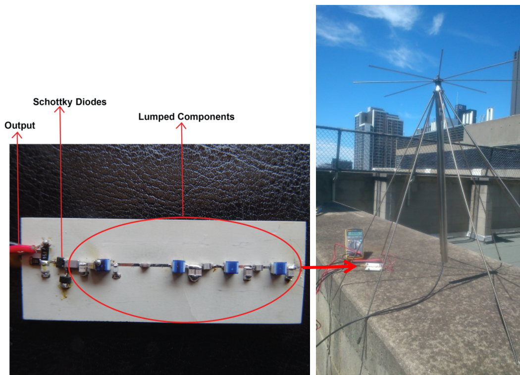
Figure 5.14 (a) Fabricated FM rectifier prototype. (b) Environmental measurement of the FM rectifier using a broadband discone antenna.
