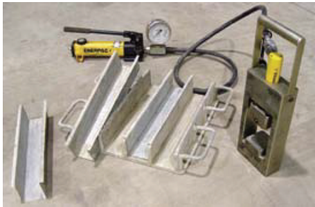
FIGURE 1: Beam end tester, showing the moulds and the hydraulic tester [18].
