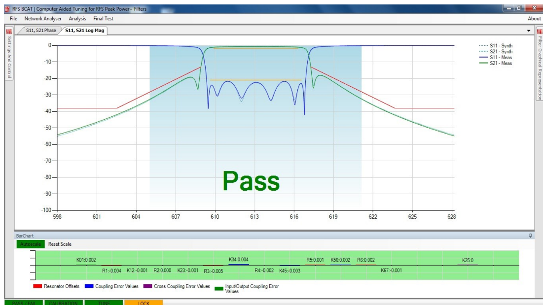
Figure 4.23 Measured filter response by BCAT while higher resolution in tuning is utilized by RoboCAT.
