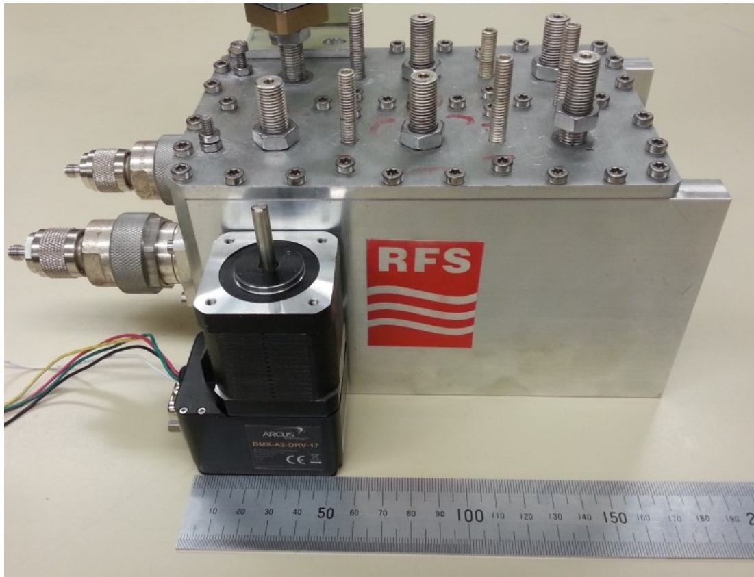
Figure 3.3 Size comparison of 6-pole cross-coupled filter and NEMA 17 actuator.
