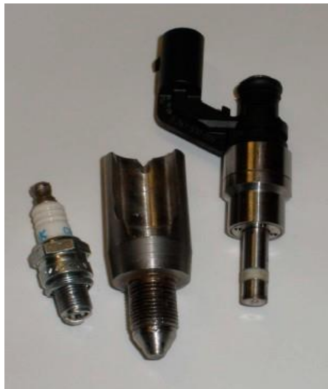
Figure 2.18 HAJI pre-chamber assembly, injector and reduced size spark plug (Boretti & Watson 2009c).
