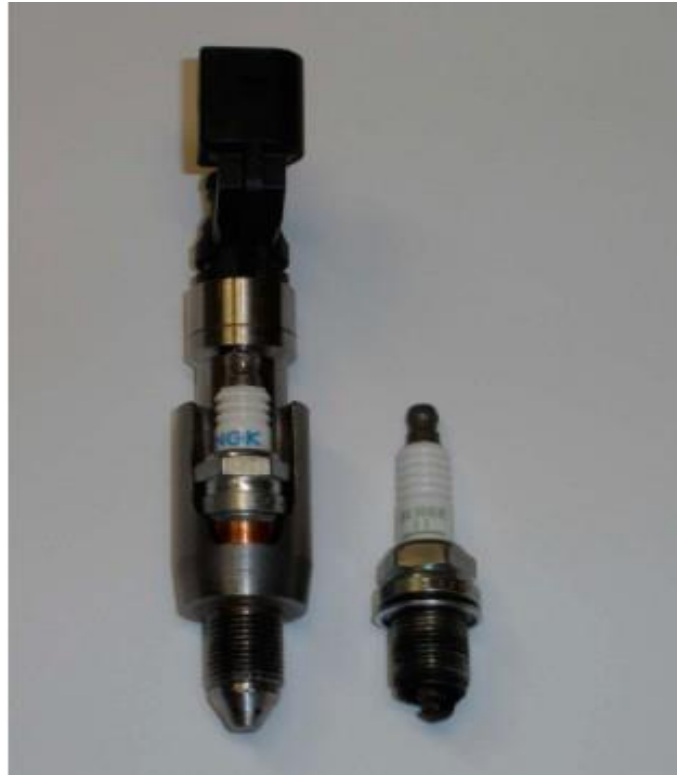
Figure 2.17 Comparison between HAJI device and standard spark plug (Boretti & Watson 2009c)
