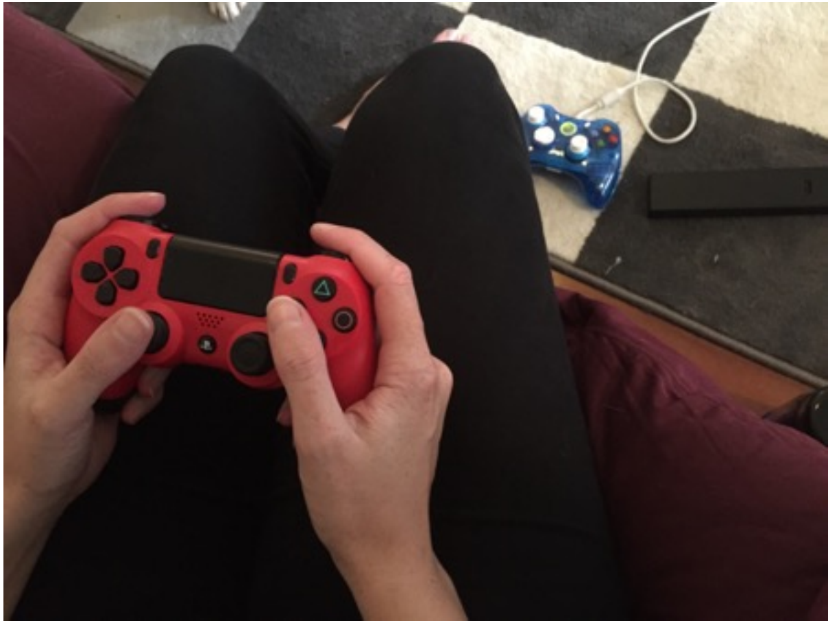
Figure 3.1. The DualShock 4, the gamepad controller for Sony's PlayStation 4 console (author's photo). On the lefthand side is the directional pad, and on the righthand side are the four action buttons (the 'X' and 'Square' buttons are currently covered by the player's thumb). Towards the bottom of the controller are the two thumbsticks (the lefthand thumbstick currently covered by the player's thumb). On the top of the gamepad, under the player's index fingers, are the shoulder buttons and triggers. The 'Share' and 'Options' buttons typically provide access to functionality external to a videogame's diegesis (such as menus), and the 'PS' button with the PlayStation logo returns the software to the PlayStation 4 dashboard. The black rectangle in the middle of the gamepad functions as both a touchpad and two further buttons (the left half and the right half), and beneath this pad is a speaker. In the background is a third-party gamepad for Microsoft's Xbox 360 console, with a similar layout.
