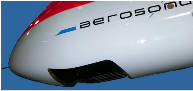
Figure 2. Payload bay of a recent variant of the AEROSONDE RPAS.
