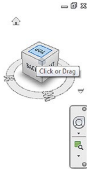
Figure 1.3 ViewCube a three-dimensional orientation indicator and controller, developed by Autodesk Research, 2008. Now Autodesk's standard orientation controller across their three-dimensional software range.
