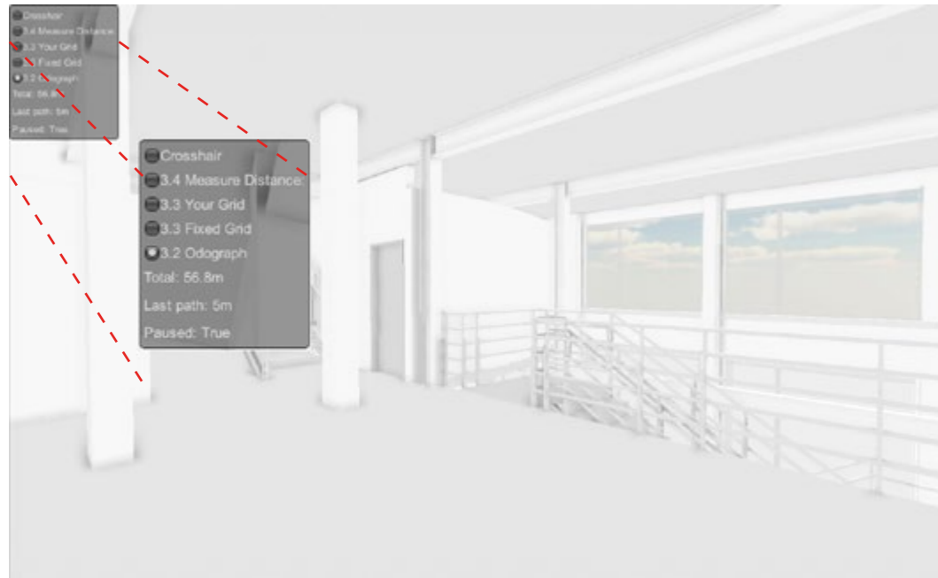
Figure 3.3.6 Odograph (2014) records and displays the user's total distance and last distance travelled, to allow correct comprehension of the scale of a building.
