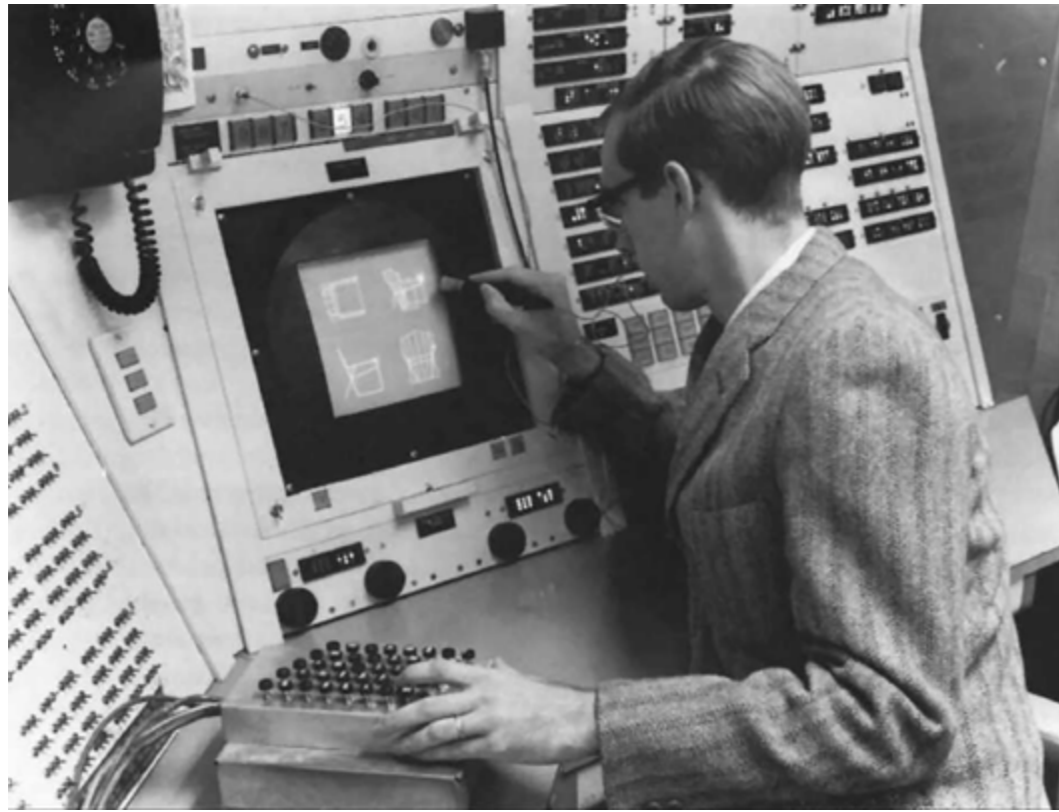
Figure 2.1.6 In a frame from the Lincoln Laboratory (1964) documentary, Timothy Johnson draws with Sketchpad's light-pen.
