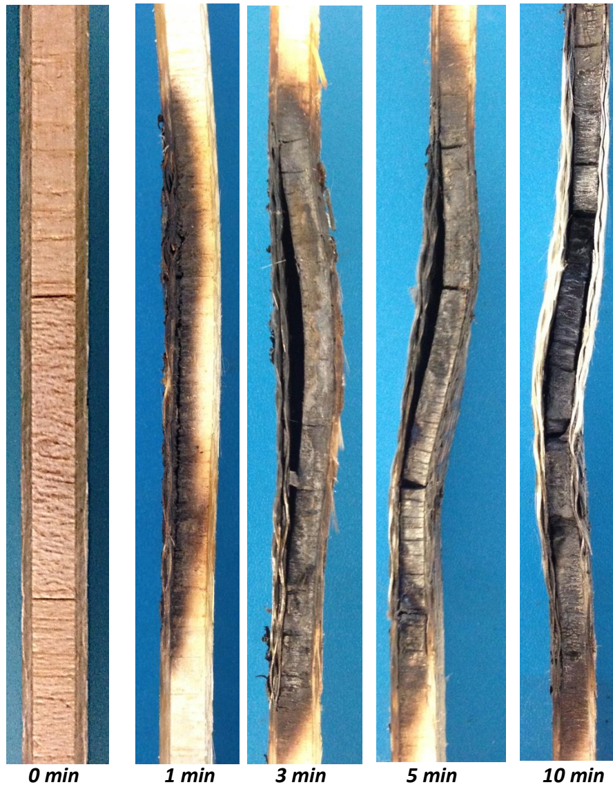
Figure 6.12: Failure modes of sandwich composites from 0 to 10 minutes heat exposure times. 0 min is a sandwich composite specimen at original condition.
