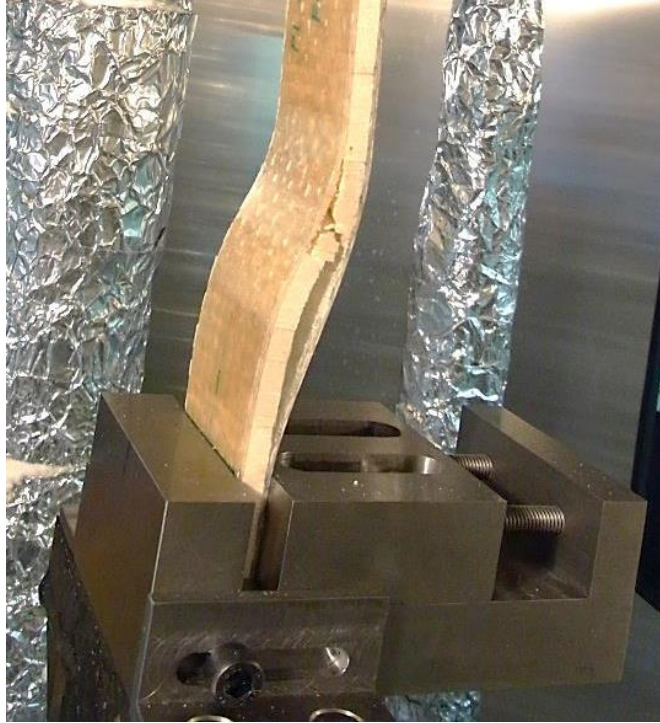
Figure 5.3: End clamping of the sandwich composite specimens for fire structural testing.
