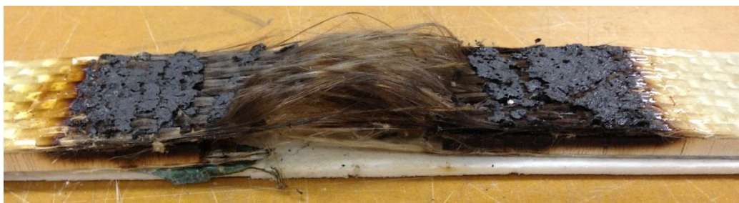
Figure 3.22: Close up view of ruptured sandwich specimen.
