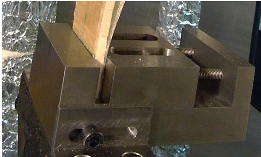
Figure 6.2: End clamped of the specimen for post-fire compression testing.
