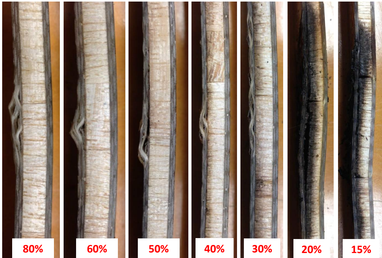
Figure 5.9: Failure modes of sandwich specimens tested at different compressive load levels as a percentage of the failure load at room temperature.
