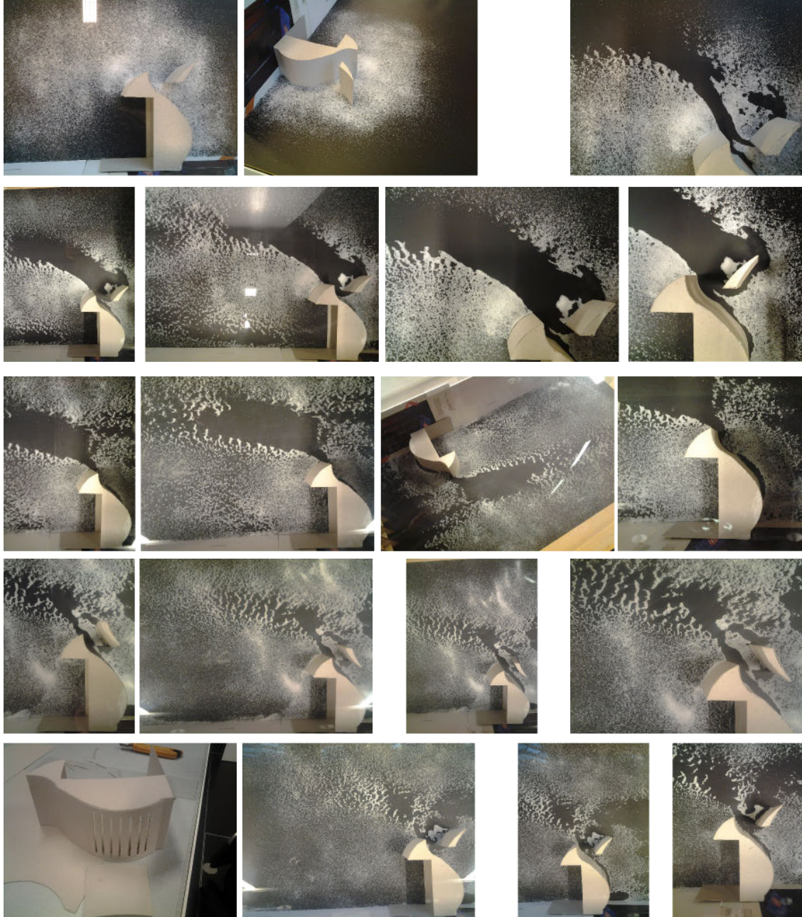
Figure 8.19: Rapid visualisation of airflow through a deflector barrier, in the mini airflow tunnel, with erosion technique. (Source: author)
