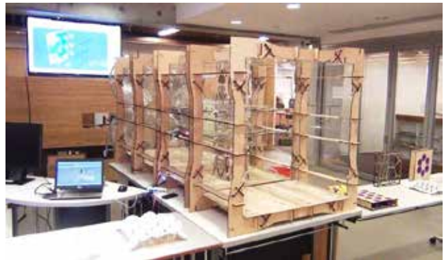
Figure 4. The assembled MWT in operation. The large screen in the background displayed the real time visualization of the sensor outputs. Several porous screen prototypes were also on display.
