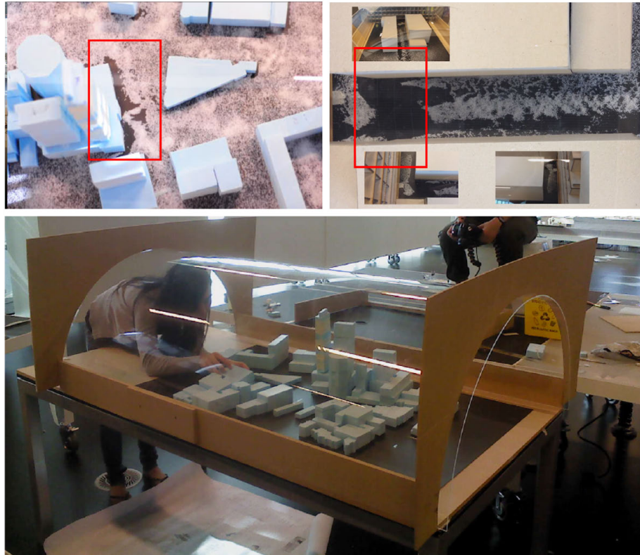
Figure 3.12: Visualisation with erosion test in the mini airflow tunnel to see the area of turbulence at the bottom of the buildings. Left: large-scale city model installation in the mini airflow tunnel. Middle: area of erosion showing the high wind speed region at the bottom of tall building. Right: experiment in the wind tunnel to visualise the wind flow and channel effect with accelerations at the corners in a space similar to a local street. (Source: author)
