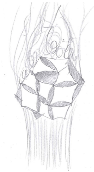
Figure 4.10: CFD visualisation of Las Piedras del Cielo (Author's sketch based on (Hermansen and Hensel 2012)). The wind is not deflected by the membranes, only a condition of porosity is observed as mitigation of wind speed.
