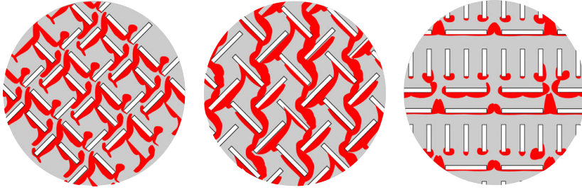
Figure 1.12: Visualisation of wind pattern through a built environment with three different building configurations. Position of buildings can prevent continuous regions of high wind speed flow. These experiments of wind visualisation were conducted in an ABL wind tunnel, using erosion technique. (Sketch elaborated by the author, based on (Beranek 1984a))
