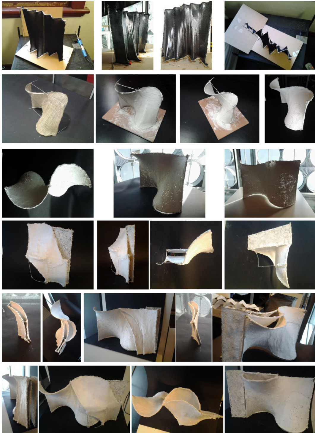
Figure 8.3: Design exploration of screens with membrane morphology. Deflectors and slot concept. (Source: author)
