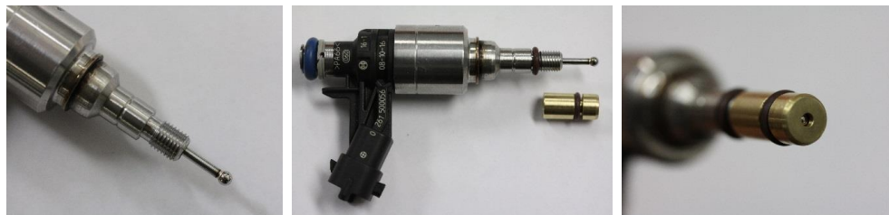
Figure 49, Modified gasoline fuel injector (left), alongside a new 2.0 mm ID brass nozzle with seals (middle) and visible sealing needle-ball.
