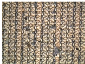
Figure 9: (a) Crack propagation in the middle of the adhesive layer and (b) top (left) and bottom(right) adherend surface from a cohesively failed surface
