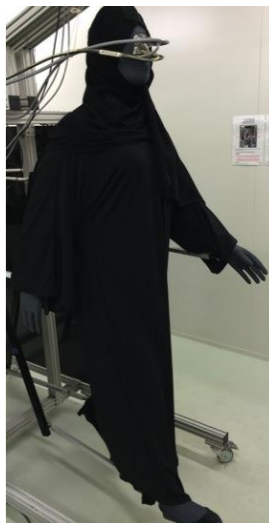
Figure 6.5 Female thermal manikin in walking mode.
