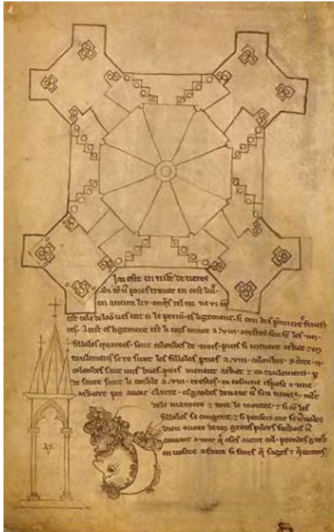
Figure 16. Page 18 from 13 th century architect Villard de Honnecourt showing the plan of a tower at Laon Cathedral and detail of a turret. 183
