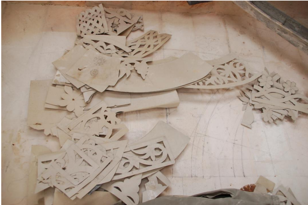
Figure 30. Stonemason templates from Midyat, Southeastern Anatolia, 2007. 311
