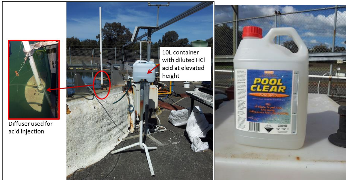
Figure 3.25 Acid injection into solar pond (right) and pool acid used for acid treatment (left)
