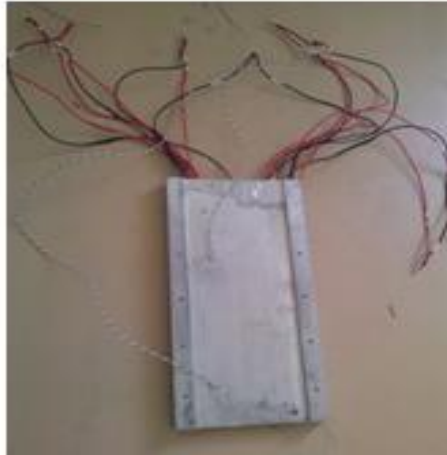
Figure 5.12 Aluminium tablet with TEG modules
