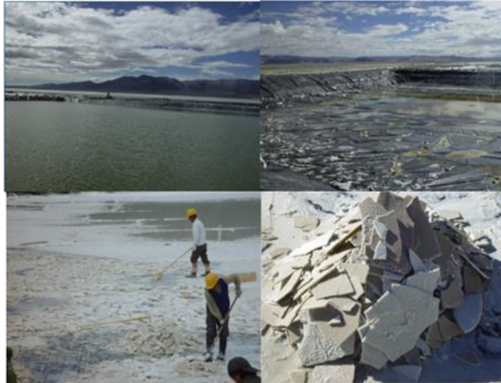
Figure 2.8 Clockwise from top left: (1) Zabuye salt lake; (2) Solar pond after evaporation; (3) Lithium Carbonate sheets, and (4) Lithium Carbonate harvesting (Nie, Bu et al., 2011).
