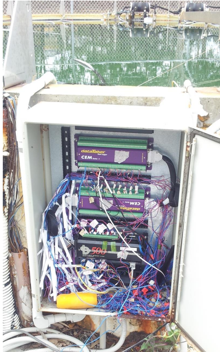
Figure 3.10 Data acquisition system for temperature and solar radiation data logging
