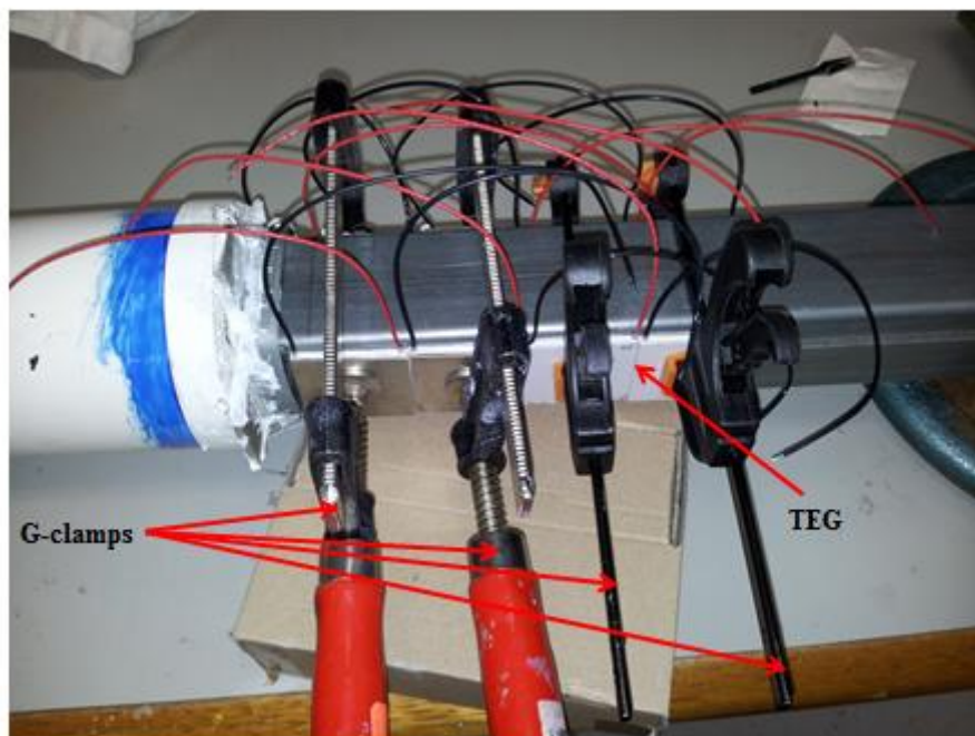
Figure 5.19 G-clamps used to attach TEGs on square channel
