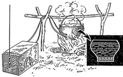
a.) Partisan's Canteen : thermoelectric generation by campfire
