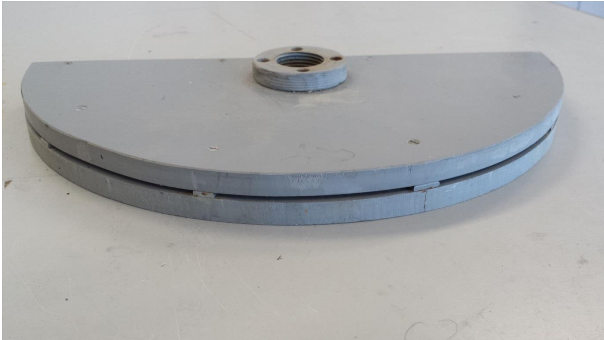
Figure 3.8 Diffuser used for gradient establishment
