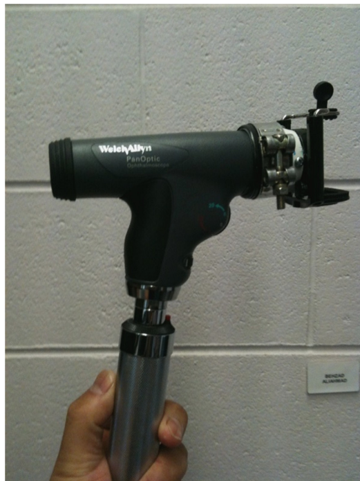
Figure 7.5 Ophthalmoscope and adjustable mount to smart phone (latter not displayed).
