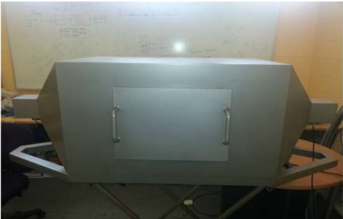
Figure 25. Fabricated custom-made TEM Cell
