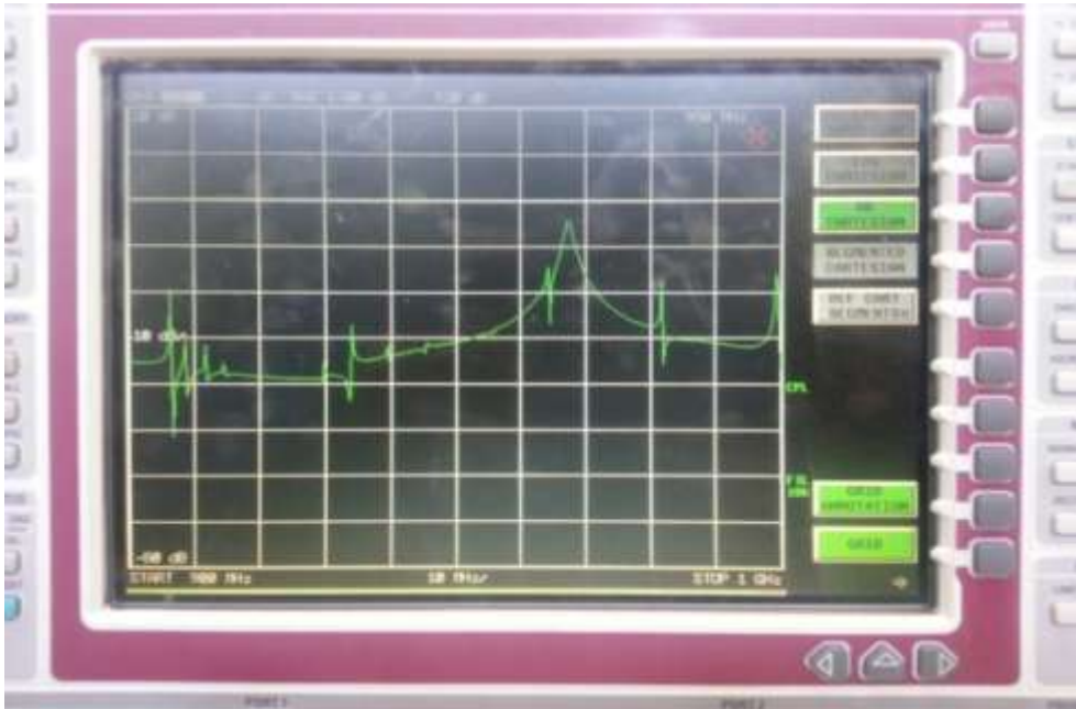
Figure 26. Ratios of waves' quantities in ch2 between b2, a1
