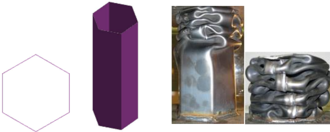
Fig. 7.3 Crumpling of Hexagonal thin walled section with 6 corner elements
