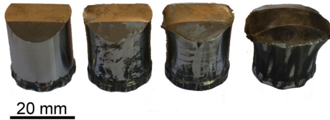
Figure 7: 20 mm FSPs from partially penetrated ballistic limit tests. Impact velocity (left to right): 365 m/s, 615 m/s, 911 m/s, 1410 m/s.
