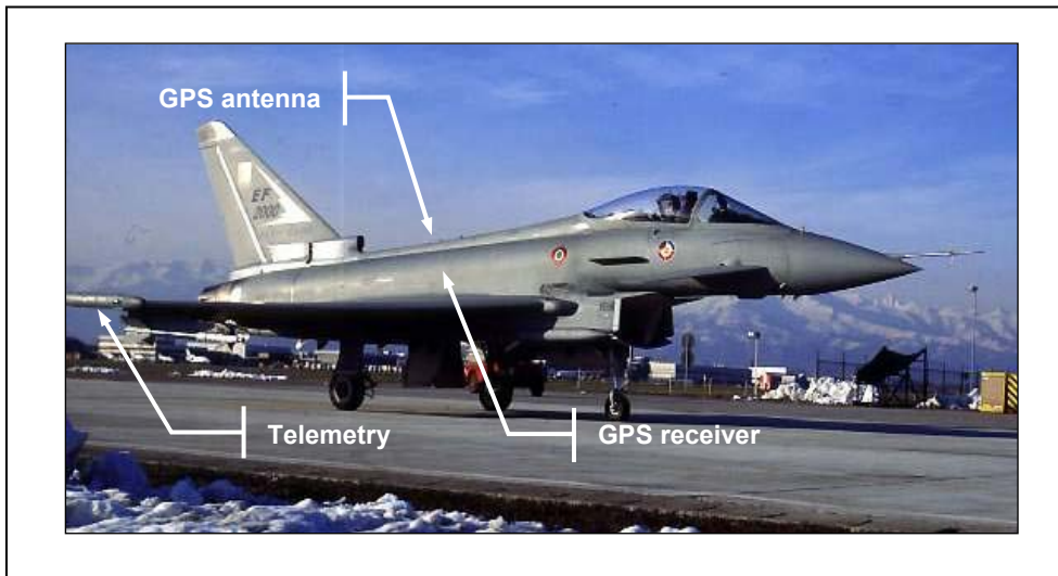
Figure 5-4: EF-2000 GPS/Telemetry Installation.
