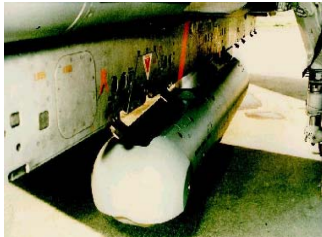
Figure 6-4: TORNADO-IDS CLDP Installation.
