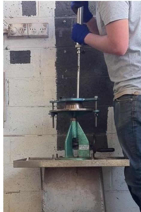
Figure 13 - Compaction into the mould on the Flow Table.
