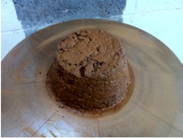
Figure 14 - The same material slightly over FMP, showing minor plastic deformation.
