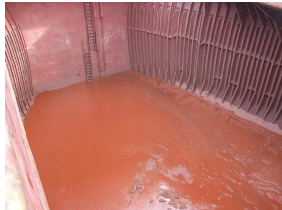
Figure 7 - Partially saturated IOF in the hold of a bulk carrier in India [25].
