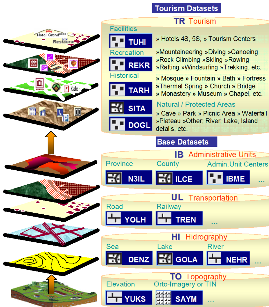
Figure 9-2 An example of datasets for a Tourism Management Information System (Aydinoglu and Yomralioglu 2007)
