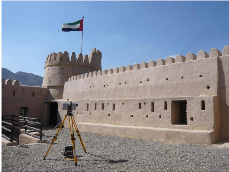
Figure 8-10 Positioning and preparation of the TLS equipment for scanning at Al Bithnah fort
