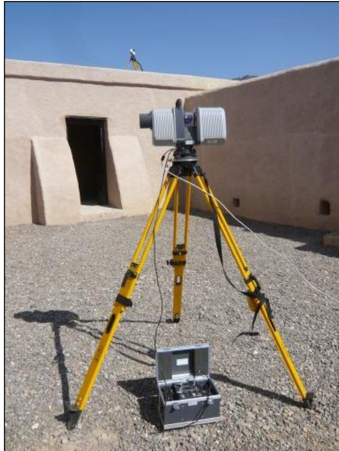
Figure 8-1 Trimble CX 3D Laser Scanner set up inside Bithna Fort, Fujairah
