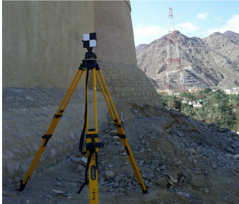
Figure 8-9 An example of control target used at Al Bithnah
