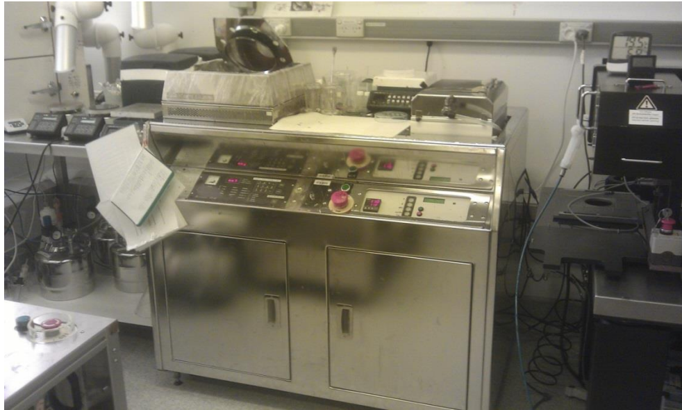
Figure 4.8: Spin coater is used to develop thin film of resin on the substrate surface. Epoxy Su-8 resin and KMPR 1025 (photoresist) have been used in this study to develop patterns on the glass surfaces and silicon wafer, respectively.
