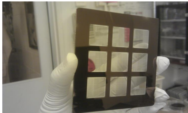
Figure 4.5: A typical photomask (dark areas are Chrome coated) of size (100 mm × 100 mm).
