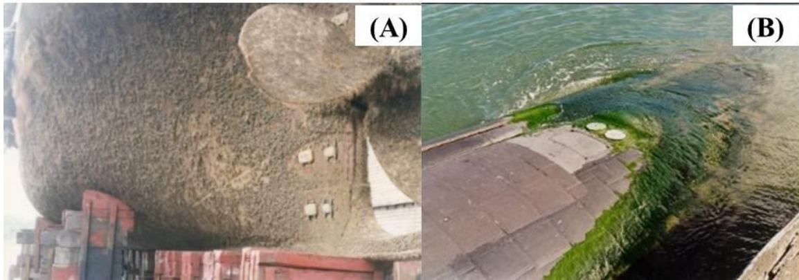
Figure 2.3: Marine vessels fouling: (A) ship hull fouling by barnacles (source: Rosehahn et al. 2010), (B) green algal (seaweed) fouling on submarine hull (source: Callow and Callow 2011).
