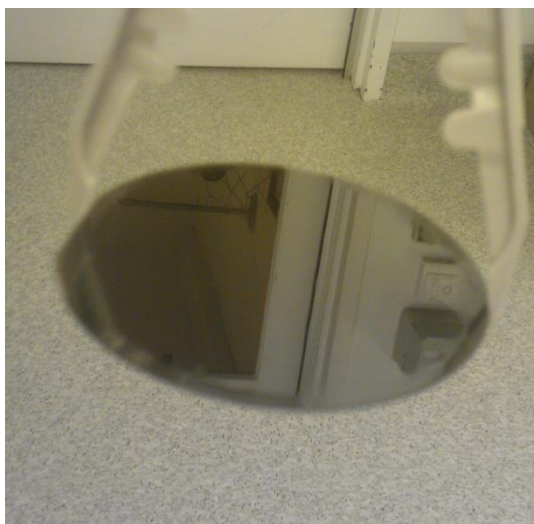
Figure 4.6: Silicon wafer (100 mm diameter) with a polished surface which is commonly used as a standard substrate in the photolithography process.
