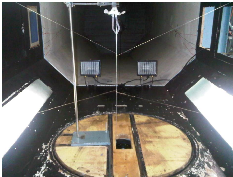
Figure 3.9: Lighting setup in the wind tunnel for high-speed imaging.
