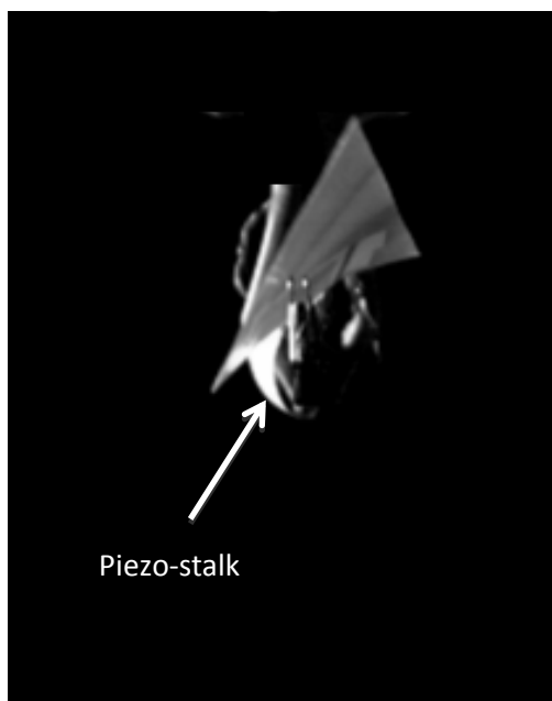
Figure 4.29: Image at 8.0m/s. Clamping strip interfering flapper motion.
