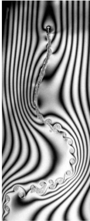
Figure 2.18: Vortex shedding at the wake of a flapping filament in a two-dimensional, parallel flow (Jun et al., 2000).
