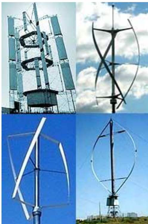
Figure 2.4: Some of the VAWT designed for urban environment. (Source: http://www.lowcarboneconomy.com )
