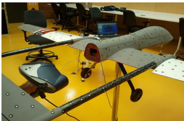
Fig. 1. 3D scanning of the JAVELIN.
