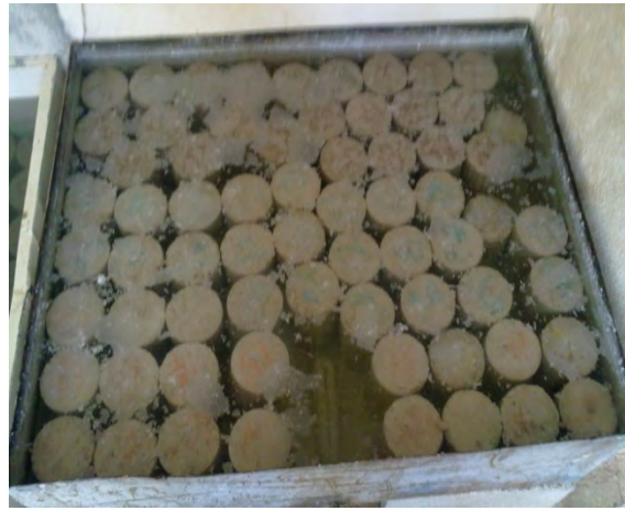
Figure 2: Specimens' curing at room temperature
