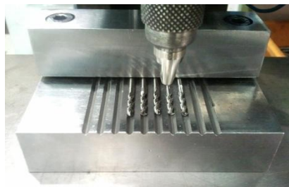
Figure 3.5. Image of the R40 stub drills held in a multiple vee clamp with the Vickers indenter above.
