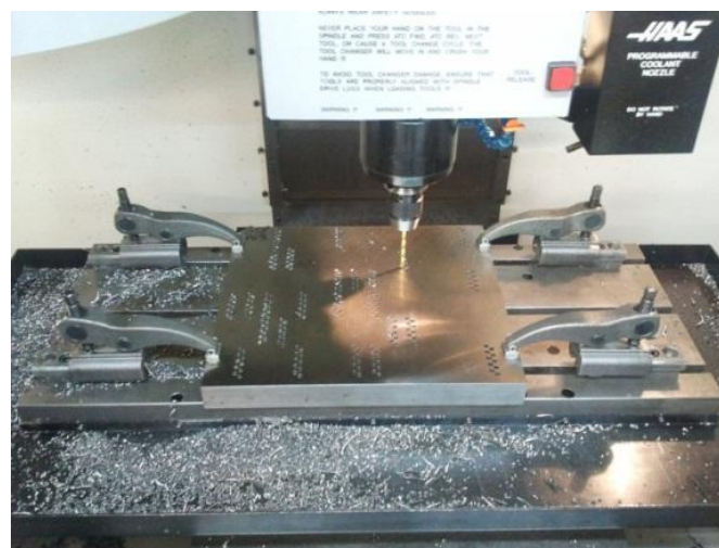
Figure 3.4. Image showing the drill test setup in a HAAS VF2 VMC.
