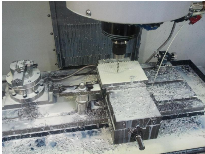
Figure 3.15. Image showing the drilling setup in the HAAS VF2SS for torque and thrust measurements, left shows the Kistler dynamometer with a D2 test piece, followed by on the right a larger D2 test piece mounted in a rigid workpiece holder.
