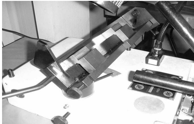
Figure 2.28. Image of the Mowhawk tool maker's microscope showing the Vee slide at a position of 90^\circ relative to the objective lens.[67]
