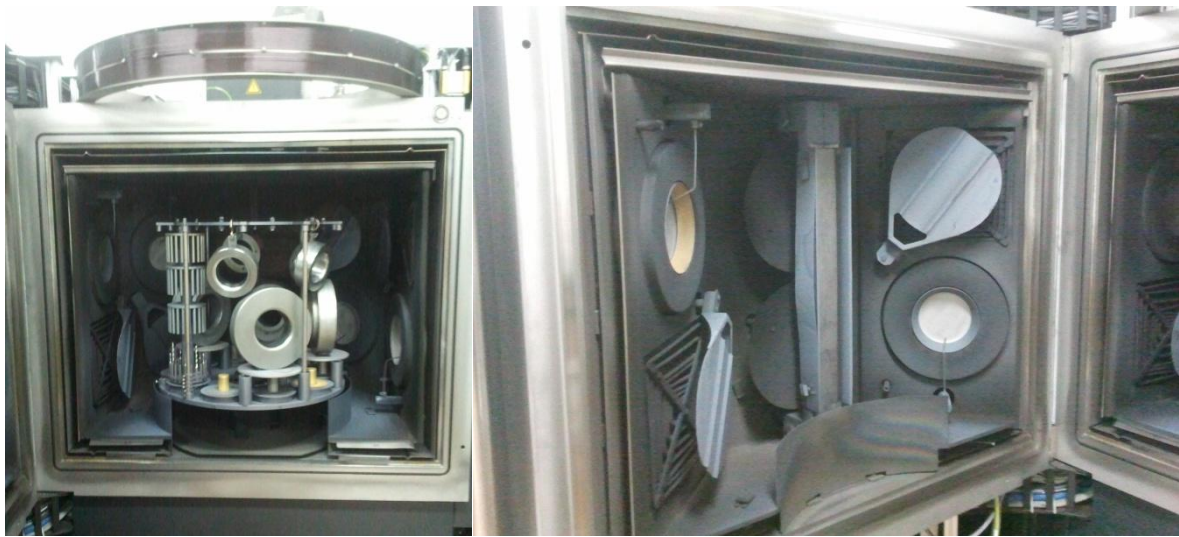
Figure 2.18. (a) Image of the cathodic arc deposition chamber used in this work (b) Chamber door with pair of cathodes and radiant heaters.
