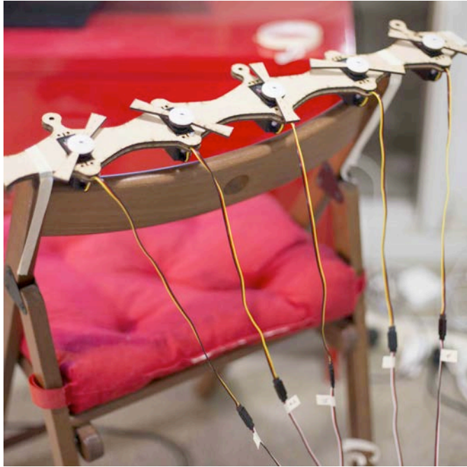
Figure 81: one of the panels of the actuator are tested before it is installed into the whole structure. This panel actuator carried five servomotors. Source: Author
