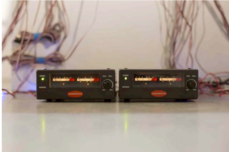
Figure 83: Power Regulators are used to regulate an appropriate current used by the servomotors. These devices prevent from overload current into the servomotor which many cases will harm or heated the servomotor. Source: Author
