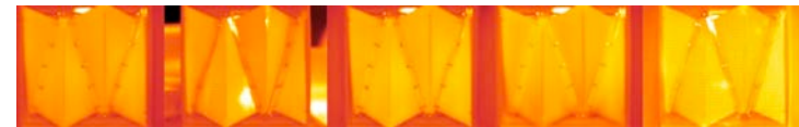
Figure 49: Images of thermal heat infrared camera located in front of the facades and the lamp heat are located in the same distance with the facades. Source: Author.
