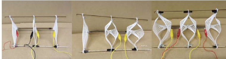
Figure 31: three component of physical prototype of Triangular are tested using smart memory alloy spring when the heat are supplied to the spring, the spring contract and pulling the two dimensional panels of triangular panels away from each other and affect the component to open. When the spring is cooling down it will return to the original state and the kinetic component return to the original state. . Source: Author.
