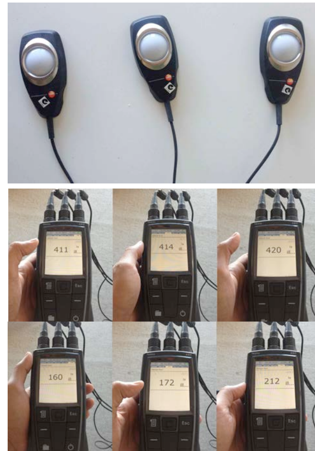
Figure 93: Three light sensors are used to measure the lighting condition taken throughout the day. The sensors are located on the floor parallel to each other, which have 1-meter distance to each other and 1-meter from the window. Source: Author.
