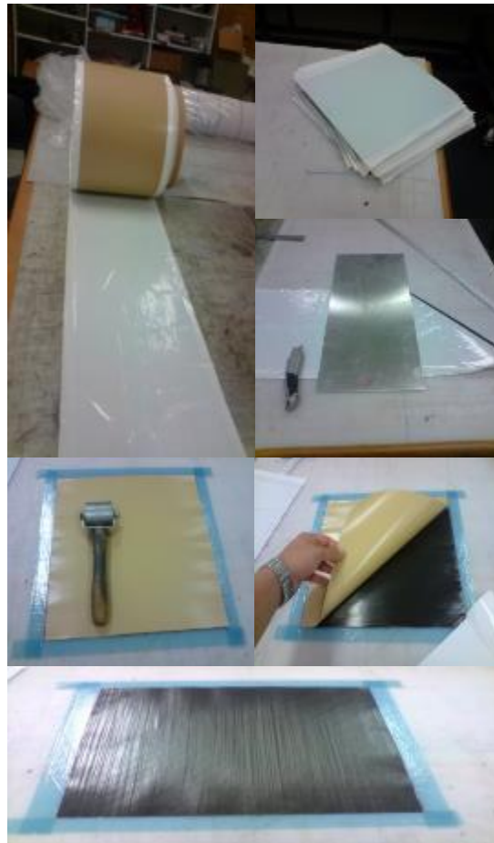
Figure 3-3: Lay-up process of carbon/epoxy laminate
