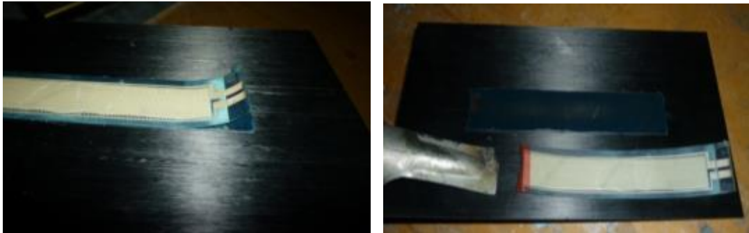
Figure 5-7: The MFC sensor is detached from the structure.
