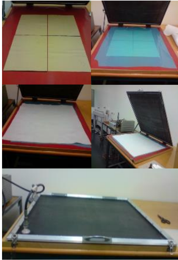
Figure 3-4: Vacuum bagging process
