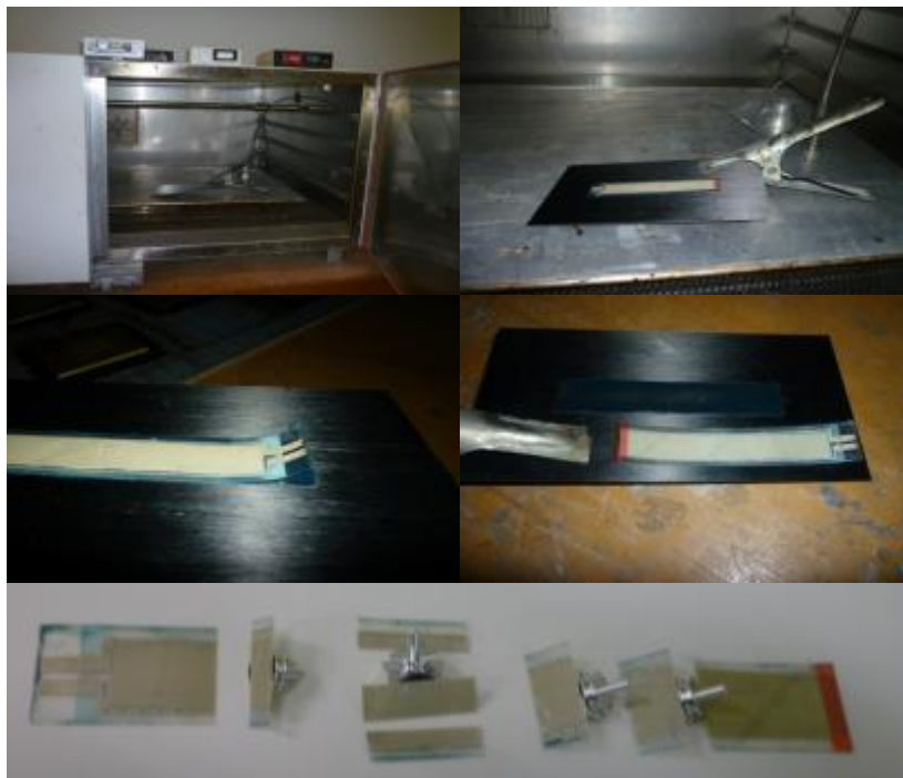
Figure 3-21: The transducer detaching process and sample preparation
