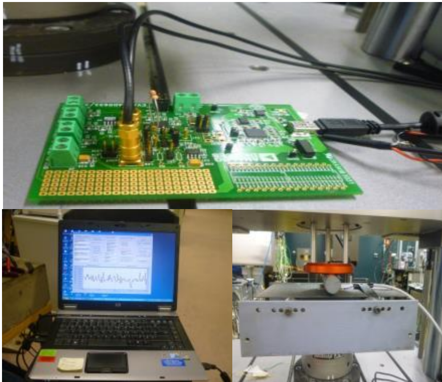
Figure 3-19: E/M impedance measurement test setup
