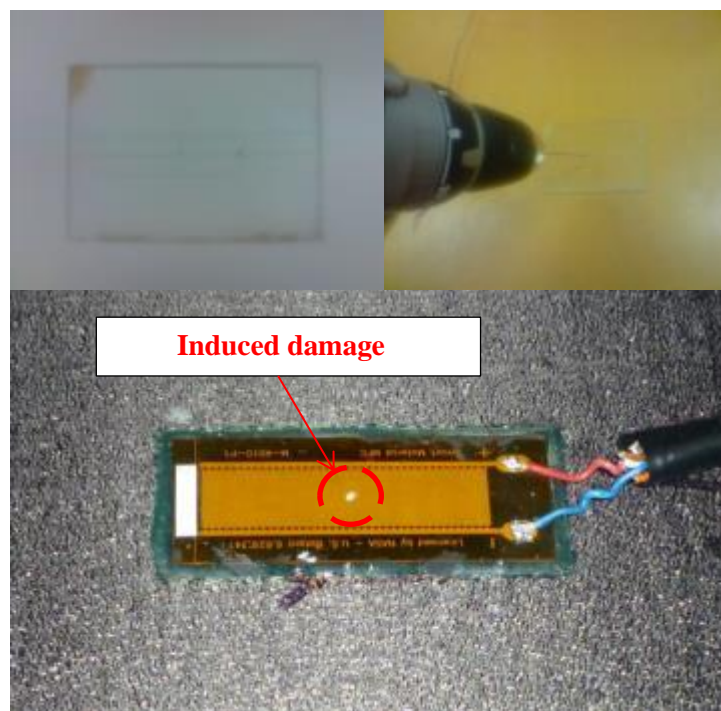
Figure 3-8: Damage induction in MFC transducer
