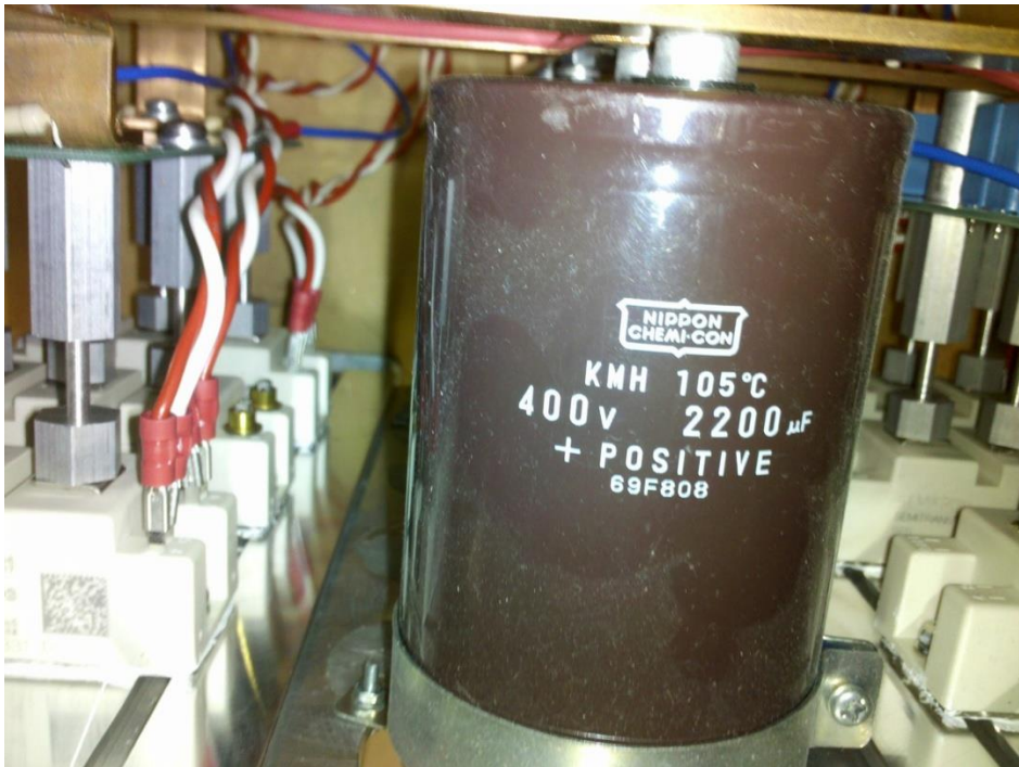
Figure 9.4: One of the 4 capacitors used as the DC link within the converter.
