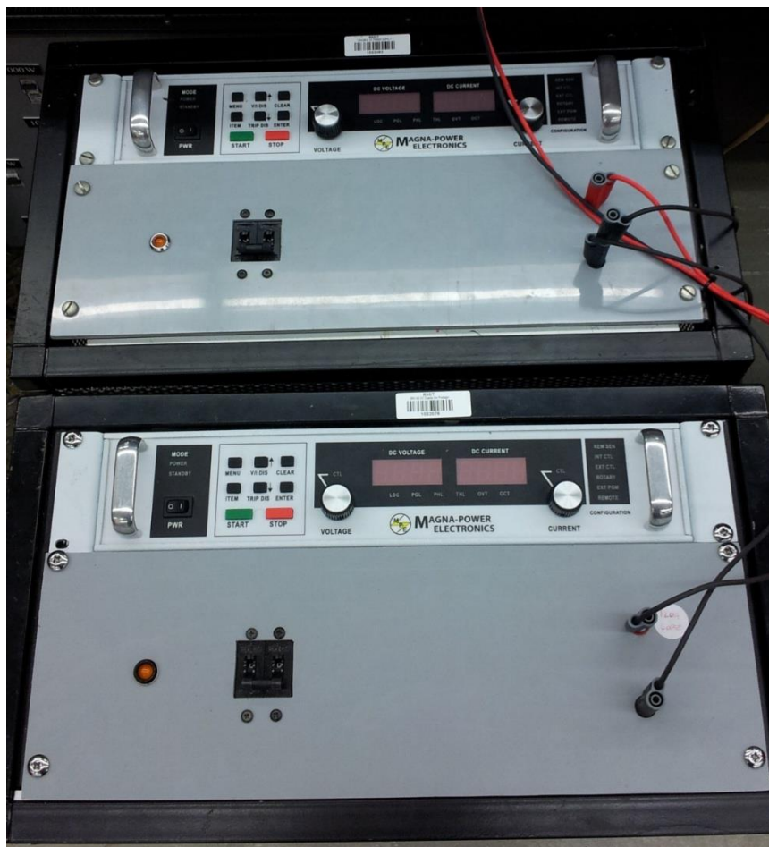
Figure 9.5: Two DC sources in series using Magna XR250-24.
