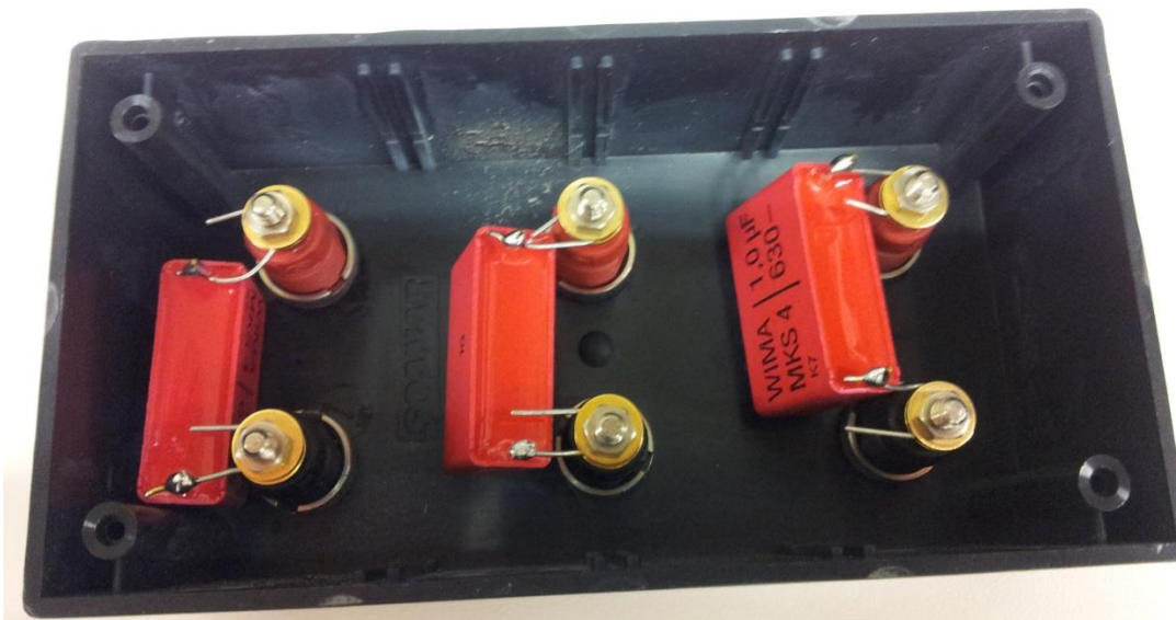
Figure 9.17: Bottom view of the enclosure of the capacitors for balance booster.
