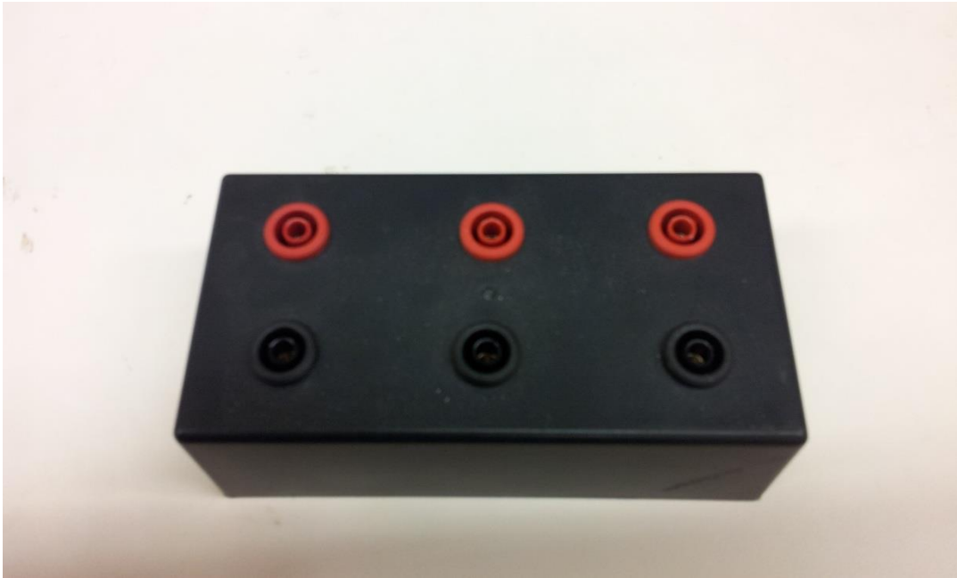
Figure 9.16: Top view of the enclosure of the capacitors for balance booster.
