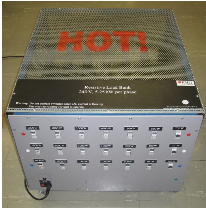
Figure 9.13: RMIT lab resistive load bank.
