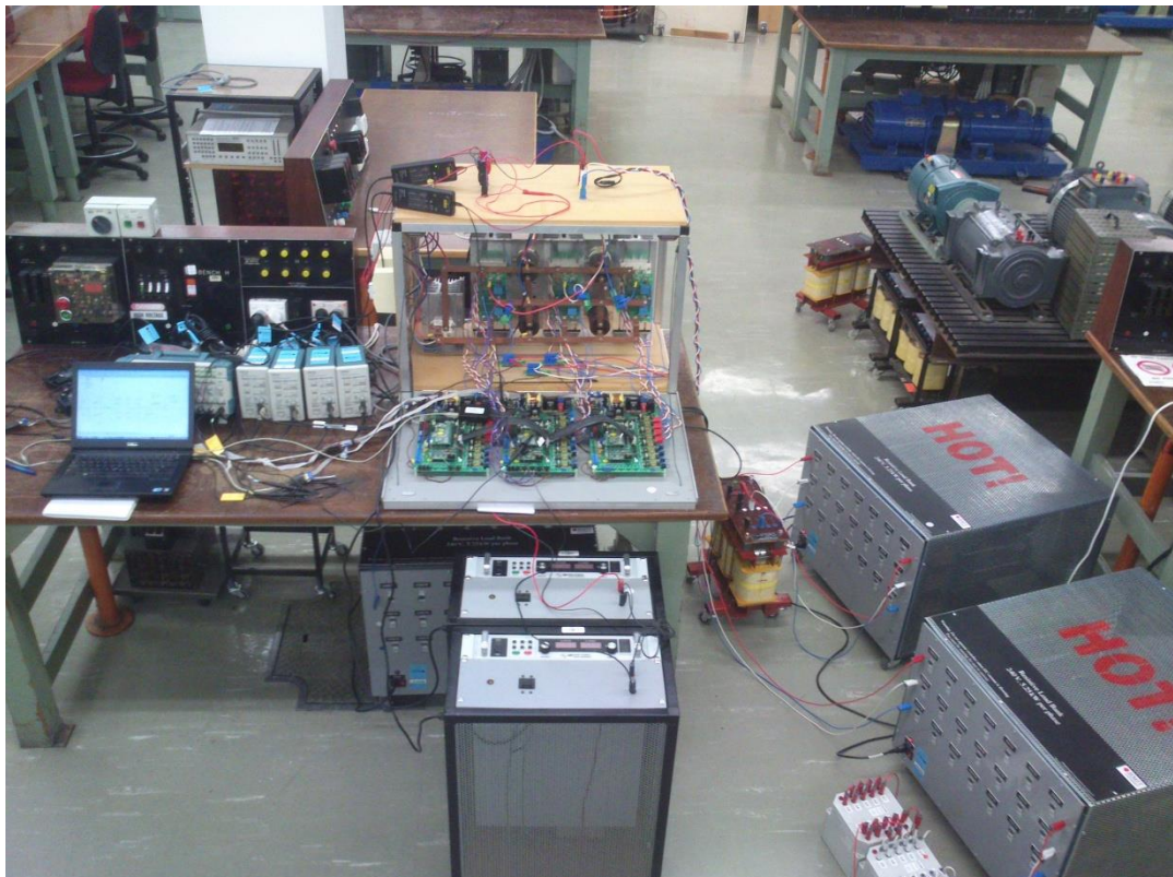
Figure 9.1: Photo of the experimental NPC converter, power supply and loads.
