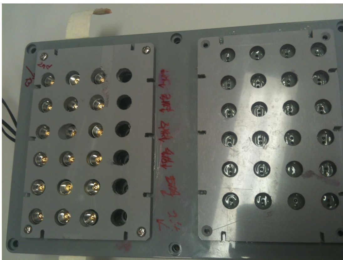
Figure 3.13: Final fabricated exposure system used for external in vitro irradiation of cancer and normal cells in this project.
