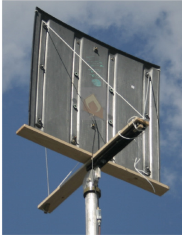
Figure 9.17: PICA antenna embedded in Adventra roof panel under test (image of the antenna overlaid to indicate position and orientation)
