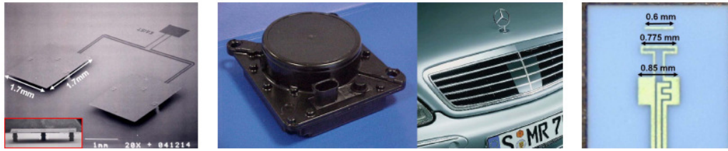
(a) a fabricated 2x1 77 GHz Patch array (b) the Mercedes Long Range Radar System (c) a 77 GHz Yagi-Uda antenna used to feed a reflector
