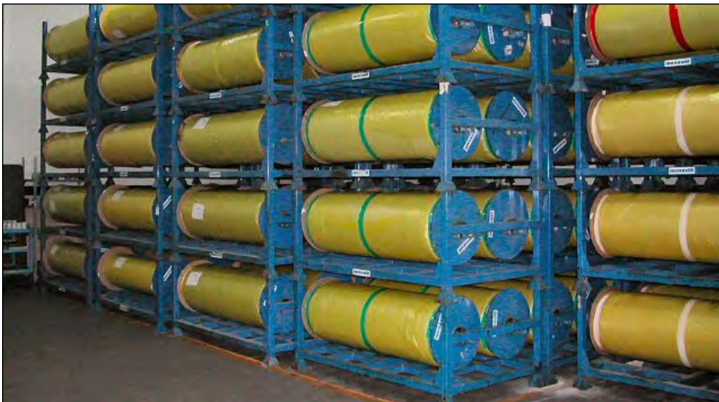
Figure 3.5: SMC storage arrangement
