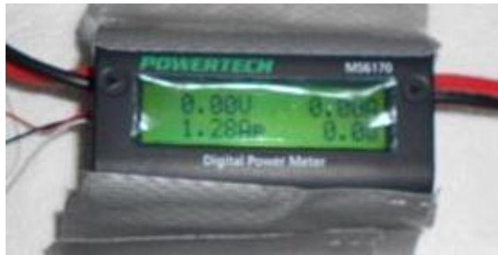
Figure 6.9: Digital DC energy meter
