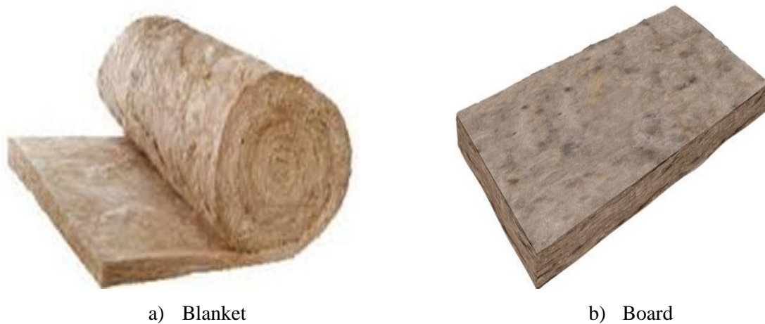
Figure 2.8: Sheep wool insulation( http://www.romansolutions.com )
