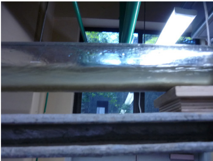
Figure 35 Photograph taken from side of the flume. Note: bed formed on the bottom of the pipe
