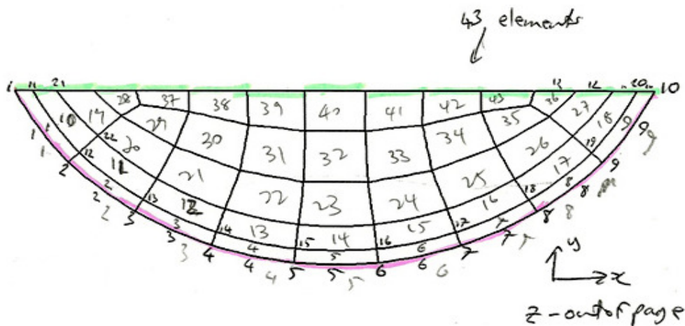
Figure 41 Sample structured 2-D mesh for 43 elements
