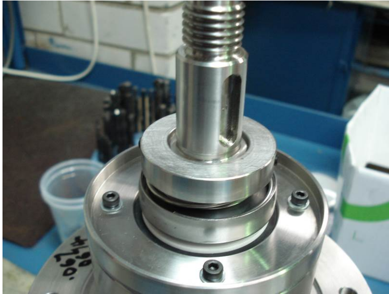
Figure 7-14 shaft and bearing housing
