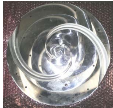
Figure 5-8 Curved nozzle profile of the turbine under investigation
