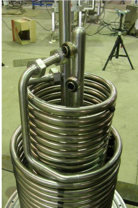
Figure 7-37 First and second layers of the condenser
