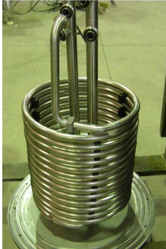
Figure 7-36 First layer of the condenser
