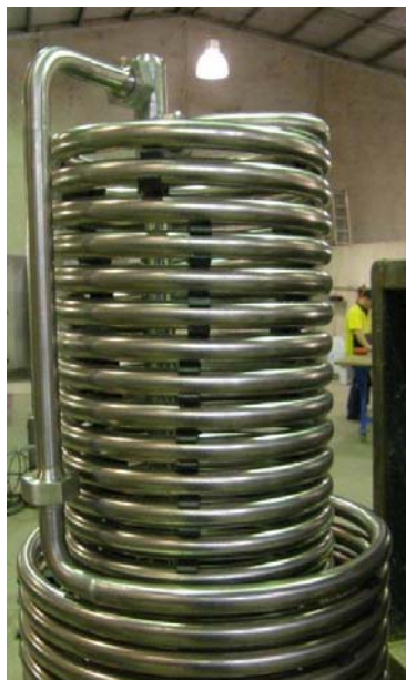
Figure 7-38 Third layer of the condenser
