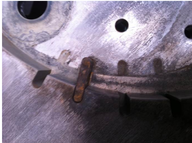
Figure 7-30 Nozzle insert and its position on the split rotor
