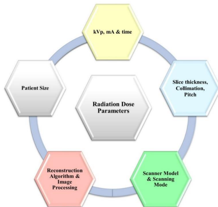
Figure 4.3 The factors of radiation dose in CT scan imaging.
