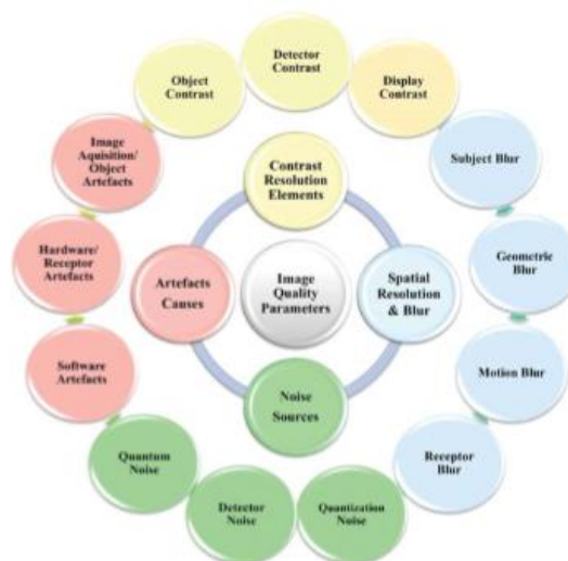
Figure 1: The parameters of image quality and the influence factors of each parameter.
