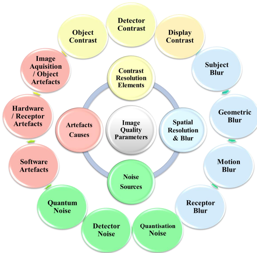
Figure 2.5 The parameters of image quality and the influence factors of each parameter.
