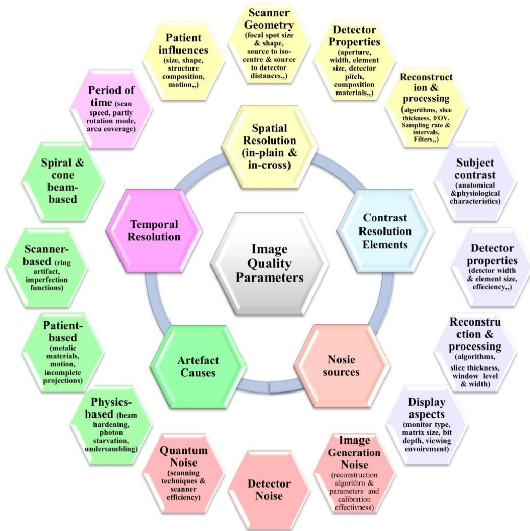
Figure 4.2 Parameters of image quality an.d the influence factors of each parameter
