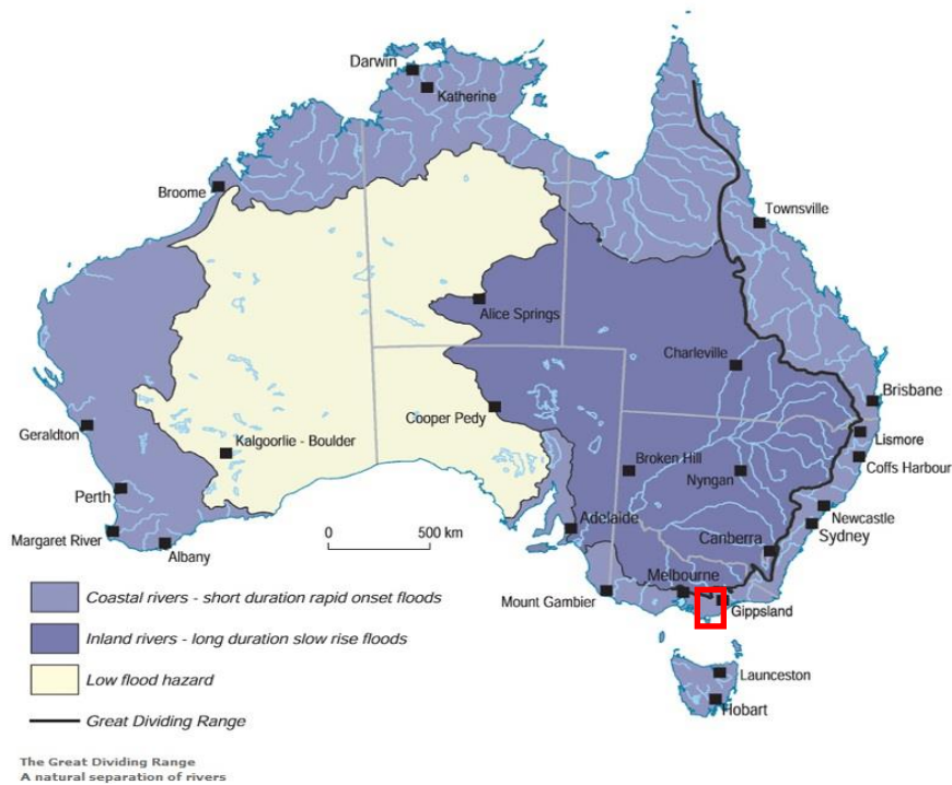
Figure 3.6: The natural separation of hydrodynamic behaviour in Australia. Red box refers to figure 3.7
