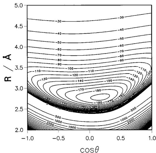
FIG. 1. Contour plot of the potential energy surface of He·NO<sup>+</sup>.
