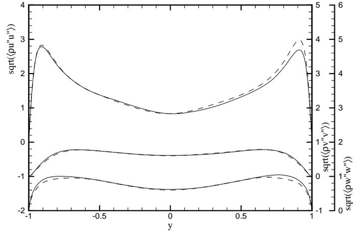
**FIG. 6.** Root mean normal turbulent stresses, comparing current simulation (dashed line) with Coleman *et al.*[14](solid line). The top curves relate to the left scale, the middle to the right scale and the lowest to the furthest right scale.
