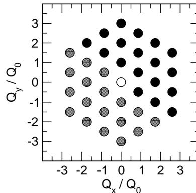
FIG. 3: Set of  $\mathbf{Q}_\mu$ -vectors up to third order (*i.e.* three “shells” around the origin) in reciprocal space used in the small-harmonics Fourier-filtered method to compute  $\rho_{\mathbf{Q}_\mu}$ . Due to the reality of  $\rho(\mathbf{r})$  we have  $\rho(\mathbf{q}) = \bar{\rho}(-\mathbf{q})$  and it is therefore sufficient to compute only half of the 36 coefficients  $\rho_{\mathbf{Q}_\mu}$ .
