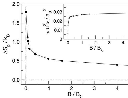
FIG. 11: Entropy jump  $\Delta S_p$  per pancake as a function of field  $B$ . Inset: Pancake fluctuation width  $\langle u^2 \rangle$  normalized to  $a_0^2$  at the melting point (the Lindemann number squared).
