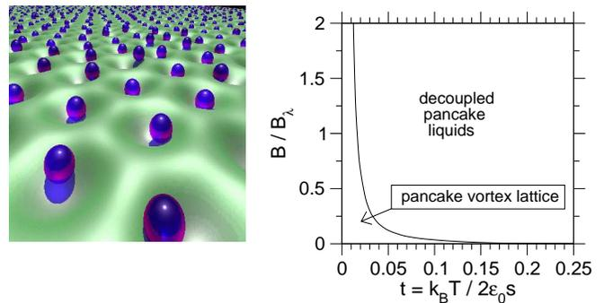
FIG. 2: Left: Snapshot of the pancakes (visualized by spheres) placed onto the substrate potential (visualized as a surface) at  $B = B_\lambda$  and  $t = 1/59 \approx 0.017$  just below the melting transition to demonstrate how the substrate potential constrains the pancake motion. Right: The phase diagram we have computed using the substrate method.
