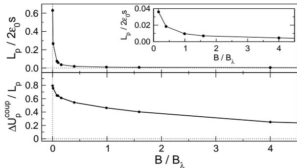
FIG. 10: *Top*: Latent heat  $L_p$  per pancake across the melting transition as a function of field. The inset shows the same data on a reduced scale. *Bottom*: Jump in inter-layer coupling energy,  $\Delta U_p^{\text{coup}} = E^{\text{coup}}$ , normalized by latent heat.
