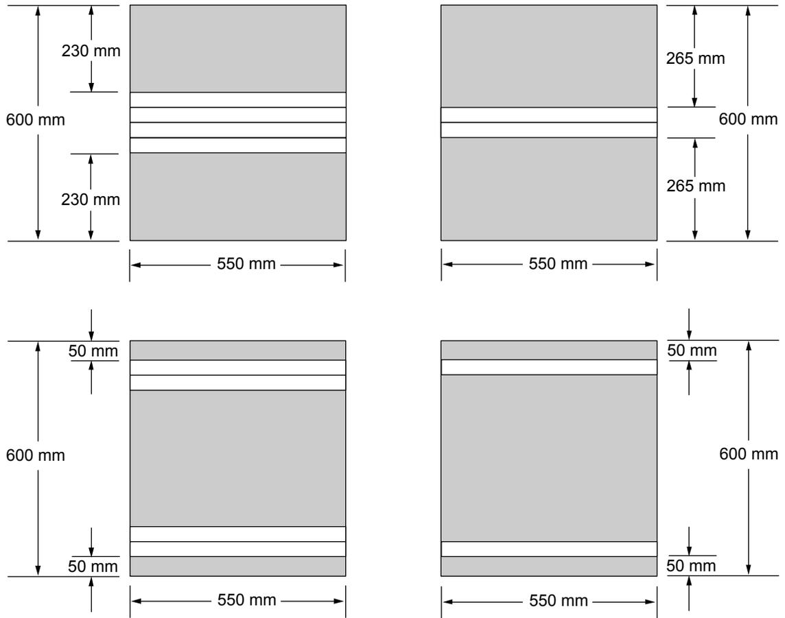
Figure 1. Diagram showing vest configurations and location of retroreflective markings.
