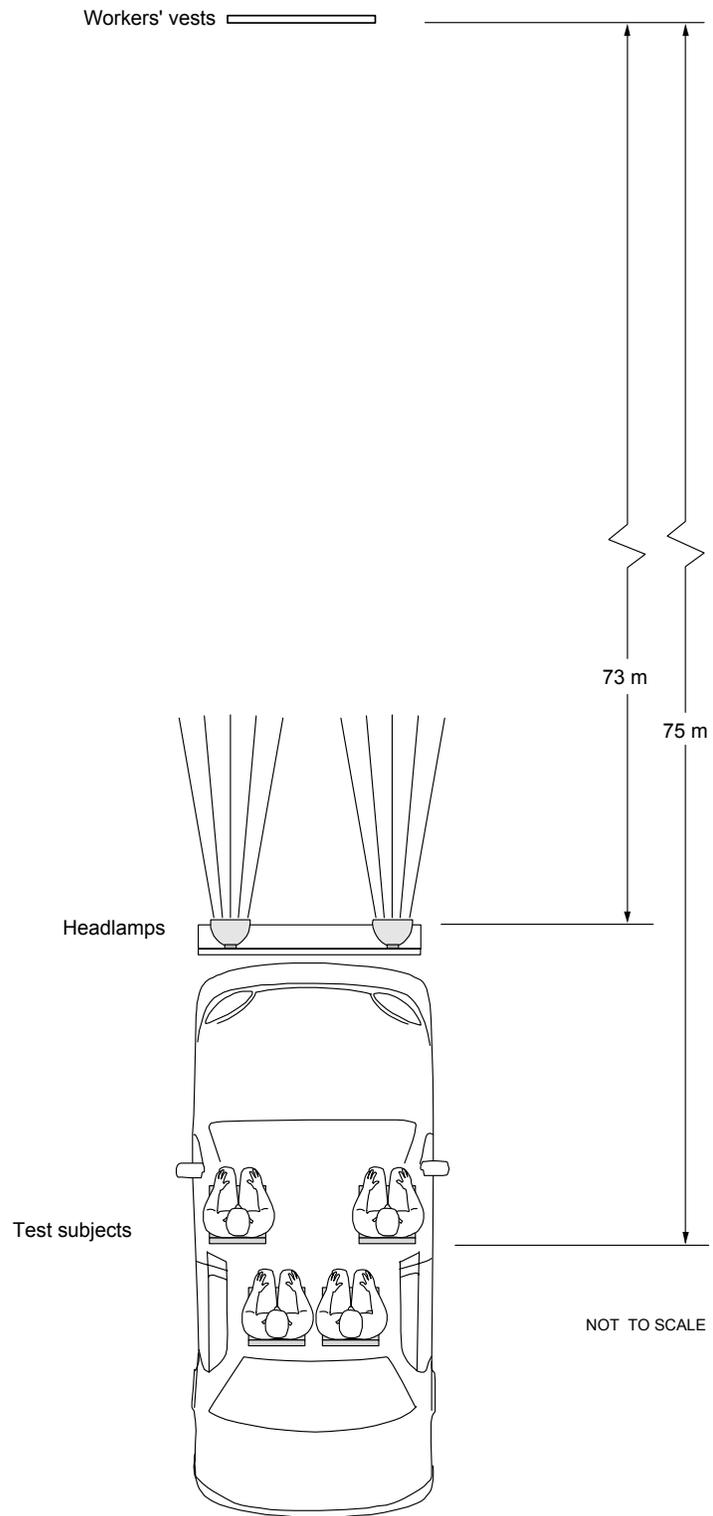
Figure 3. Overhead diagram of the experimental setup.
