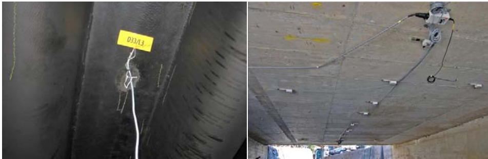
Figure 1: Strain gauges installed on a steel orthotropic-deck bridge (left), and a typical strain transducer set-up on a reinforced concrete bridge (right).
