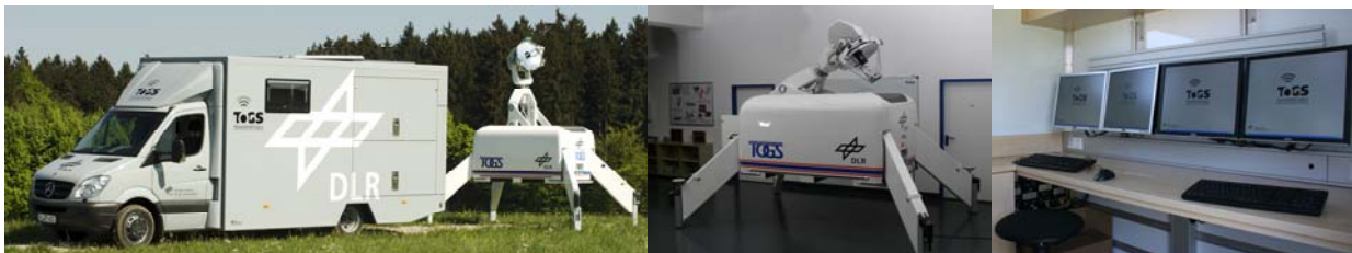
Figure 2.1. TOGS with its transport van (left), TOGS in folding process (middle), and operation room inside the van (right). Source: DLR.
