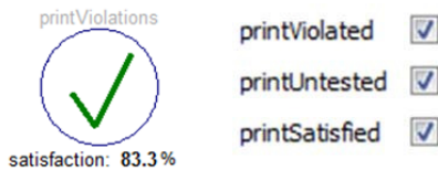
Figure 4. Defining requirement status log (left figure: icon; right figure: parameters of the block)
