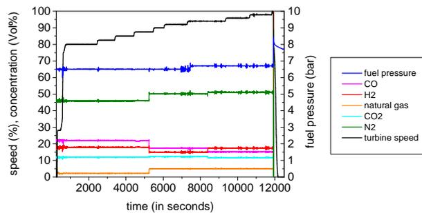
Figure 2: Fuel composition, fuel pressure and turbine speed of the turbine during operation
