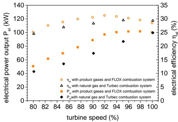
Figure 6: Steady-state operating performance of the Turbec T100 with two different combustion chambers and fuels
