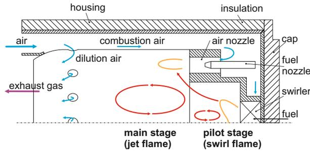
Figure 3: Schematic of the developed FLOX-combustion system
