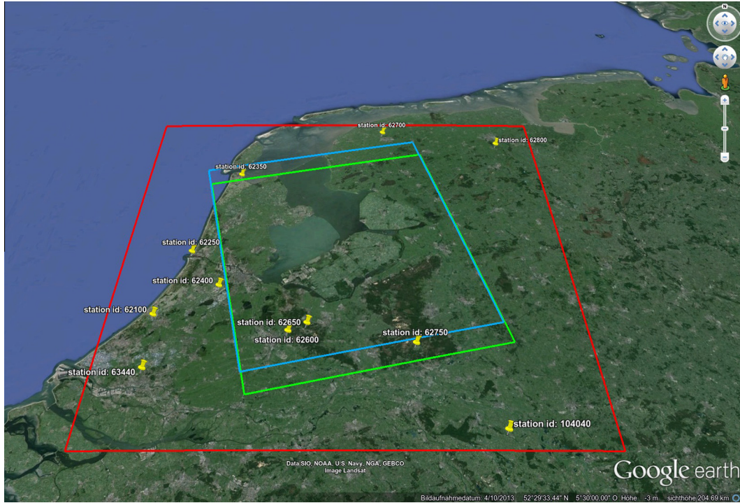
Fig. 1. Illustration of test site. The outer rectangle is the finest domain of NWP while the inner rectangles illustrate the SAR coverage of the acquisitions on 3rd and 4th October 1995. Weather stations are illustrated by yellow pins. The DInSAR image corresponds to the intersection of inner rectangles.
