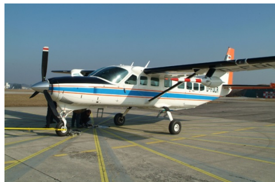
Figure 5: DLR Cessna 208B Grand Caravan with the MET-POD mounted underneath the left wing.
